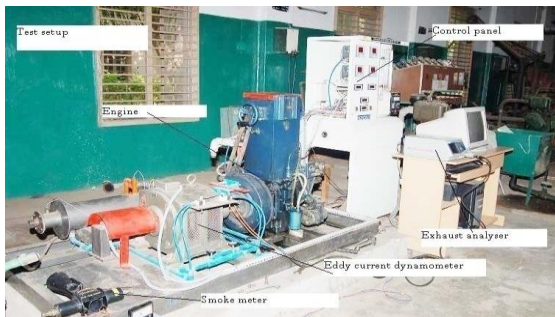
Plate 3.1 Overall view of the experimental setup
