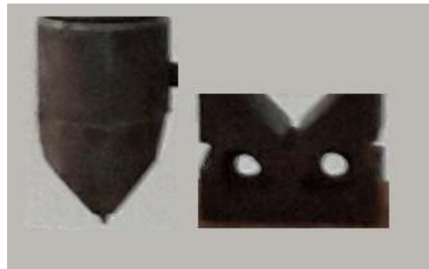
Figure.9 Fixture for short beam test
