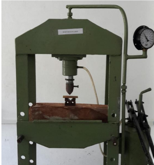
Figure.10 short beam test setup
