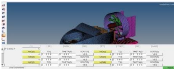
Fig.11. Ply thickness and ply orientation
