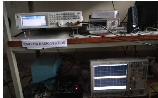
Fig. 4. 107 MHz NB-IoT Base station designed at 5G_IoT Lab, ECE Department, SMIT
