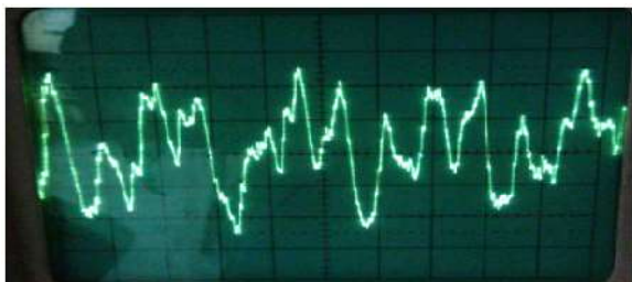
Fig.4.Input Voice Signal Waveform Obtained InOscilloscope
