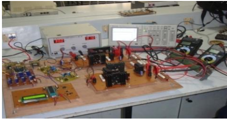
Fig 8. Hardware setup of multiple dc-dc converter in ISOP configuration with closed loop
