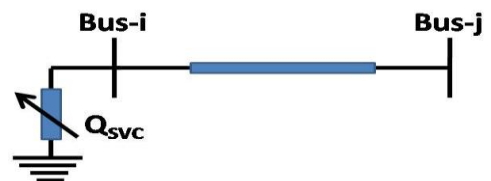
Fig.1. Mathematical power injection modeling of SVC
