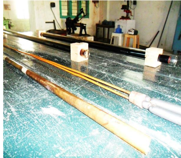
Figure 1 : Experimental Set-up for thermal performance analysis of evacuated U-tube solar collector-
