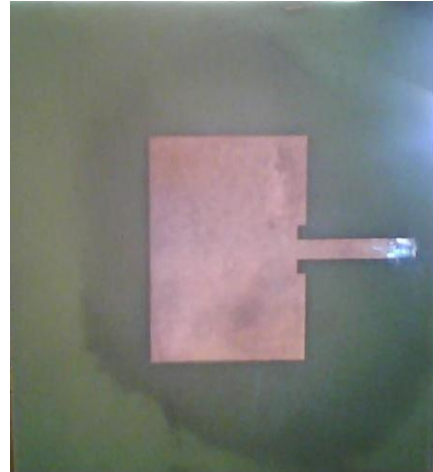
Figure 2- Fabricated model of the proposed antenna
